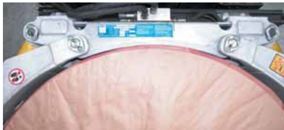
Above: Contoured frame minimizes contact pressure and potential of bruising paper. Right: RSQ with optional Flexi-Pad.
