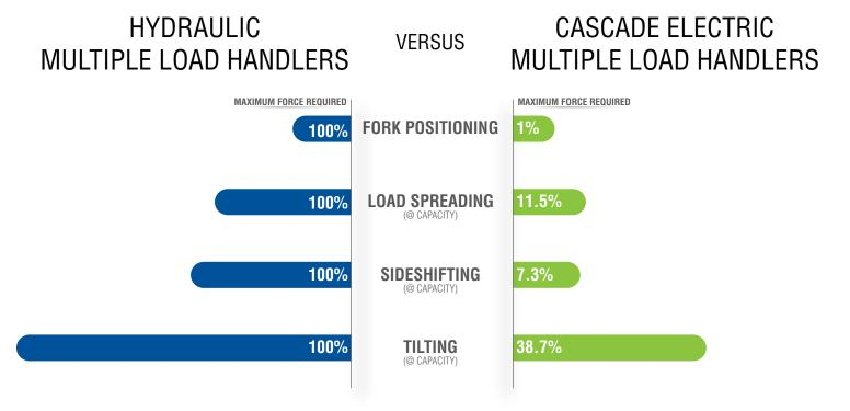
Electric MLH requires less force than a standard hydraulic MLH minimizing energy and resulting in significant energy efficiency.
