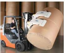
**SINGLE, MEDIUM TO LARGE ROLL** 45F, 25H, 30H, 33H, 72G, 77F, 90F, 100F — Designed for mills, warehouses, corrugators and converters handling kraft, linerboard and coated papers.
