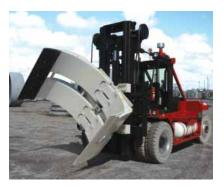
JUMBO, BIG ROLL 120F, 130F, 70H, 150F, 160F, 120H — High production roll clamp for wide printing paper handling of kraft, linerboard and coated stock.
