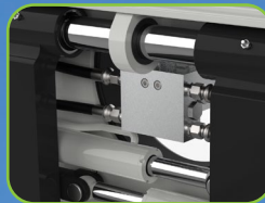
Added durability with chrome plated cylinder rods and shaft
