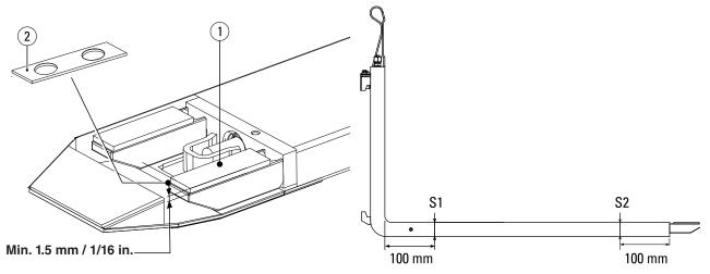
The thickness of Wear Strips (1) may not be less than 1.5 mm (1/16 in.). When Wear Strips (1) have worn to this thickness, replace them or fill with spacers (2). See point 3 of the Maintenance Schedule."
