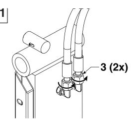
Screw the hose connectors (3) tight. **Tools required:** Open-ended spanner 22.
