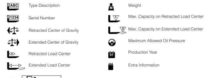
**WARNING:** Never exceed the maximum truck capacity as seen on the truck type plate. Rated capacity of both truck and attachment is the responsibility of the truck manufacturer and may be less than the capacity shown on the attachment type plate.
