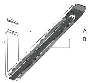
When surface A (dark grey, integrated wear plate) is worn to the extent that it is level with or below surface B (light grey), then the sleeve (1) must be replaced or fitted with a welded-on wear plate. For more information about welded-on wear plates, please contact your fork supplier. See point 4 of the Maintenance Manual.
