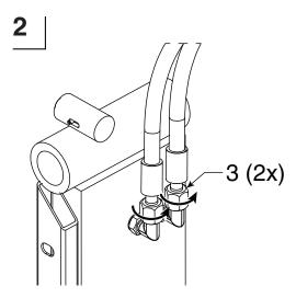
Loosen the hose connectors (3) slightly so that the pistons do not create a vacuum when removing the hydraulic parts.
