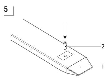
Tap the clamping bush(es) (2) into the (new) sleeve (1). **Tools required:** Hammer
