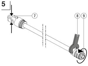
Clamp the piston rod at the rod end (7), not on the piston rod itself to prevent damage (see step 4 in this chapter). Use a size 19 (8) open-ended spanner to loosen the piston (9). If the piston cannot be loosened, heat the piston with a burner.
