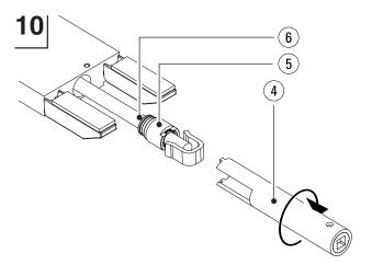
Smear Copaslip<sup>2</sup> onto the thread of the cylinder head (5). Line up the hydraulic set (6) with the cylinder and use a hammer to tap it carefully into the bore. Screw the cyclinder head tight using the cyclinder head spanner (4) and a torque wrench. See table below for torque value.
