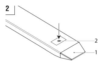
Tap the clamping bush (2) out of the sleeve (1). **Tools required:** Hammer, punch  $\emptyset$ 10.
