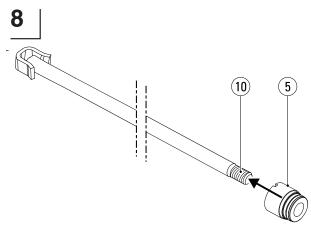
Slide the (new) cyclinder head (5) onto the piston rod (10).
