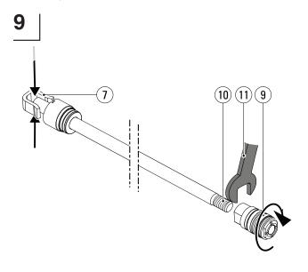
Apply loctite 270 to the thread (10) of the piston rod. Clamp the piston rod at the rod end (7), not on the piston rod itself to prevent damage (see step 4 in this chapter). Clean the piston thread with Loctite 7063. Use a torque wrench 19 (11) to tighten the piston (9) onto the piston rod (10) to a torque of 40 Nm.
