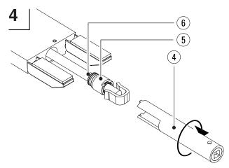
Pull the entire hydraulics set (6) consisting of the piston, cylinder head and piston rod out of the fork.
