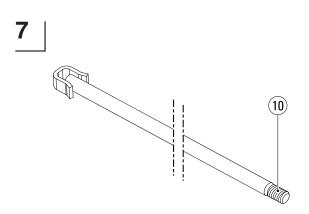
Remove remaining adhesive from the piston rod thread (10), then clean the piston rod and thread (10) using Loctite 7063.1
