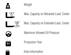
**Warning:** Never exceed the maximum truck capacity as seen on the truck type plate. Rated capacity of both truck and attachment is the responsability of the original truck manufacturer and may be less then the capacity shown on the attachments type plate.
