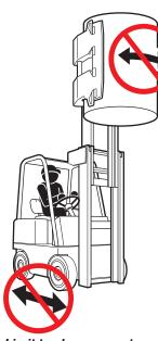
Limit truck movement with raised load.
