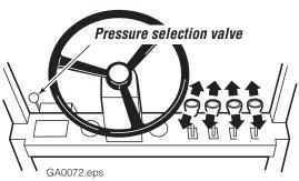
Use proper clamping force for load being handled
