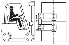
Split-Arm Clamp is recommended to handle two loads (see Handling Basics). Handling two loads with Single-Arm Clamp may be dangerous and lead to serious injury.
