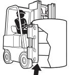
Use caution when handling unitized (wrapped) multiple stacked loads with Single-Arm Clamp.
