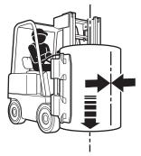
Make sure load is centered and secure prior to lifting and traveling.
