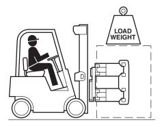
Load weight must not exceed combined truck/ attachment capacity (see truck nameplate).
