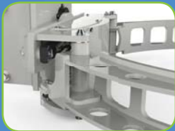
Self-lubricated arm cylinder bushings eliminates the need for grease
