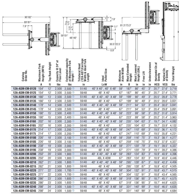
Cascade trilateral head and Mast offering is based on sit-down counter-balanced forklifts with capacity range of 6,500 lb to 7,500 lb.
