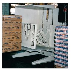
Palletizing solutions provide a reliable, economical and efficient means of inverting loads and handling pallets. Stationary Load Invertors easily transfer product to pallet/slipsheet for freezer spacer removal, damaged pallet exchange or damaged carton replacement. Load Transfer Stations quickly remove loads from pallets to make them available for transfer to slipsheets, less expensive shipping pallets, customer pallets or directly to Push/Pull platens.
