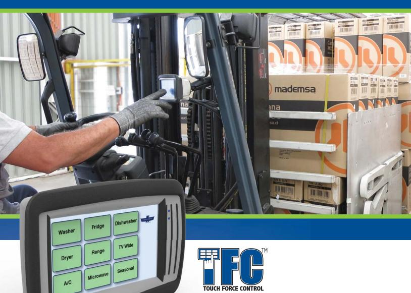
TFC is a clamp force control system that allows drivers to easily select the product being handled which then automatically applies the appropriate clamp force. The system is targeted towards operations using Cascade Carton Clamps to handle loads with different packaging types, box integrity, load size or weight. TFC is also suitable with Cascade Paper Roll Clamps, Cascade Layer Pickers or any application where regulating clamp force is required.
