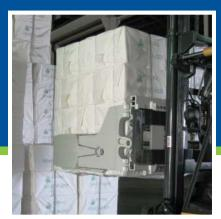
**Pulp Bale Clamps** For high-volume, damage free and secure handling of pulp bales and unitized pulp in stevedoring, mill, warehousing, shipboard and transporting operations.
