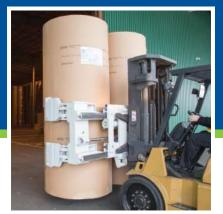
*Sliding Arm Paper Roll Clamps* When arm thickness is an issue, Sliding Arm models offer a constant narrow clamp arm profile.
