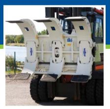
*Jumbo, Big Roll Clamps* High-production roll clamp for wide printing paper handling of kraft, linerboard and coated stock.
