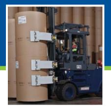
*Single & Double Tower Clamps* Designed for mills and stevedores where multiple roll handling is essential. Handle from two to eight rolls of newsprint, coated stock, kraft or linerboard.
