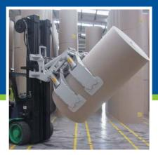
**Roll Upenders** Tilts the roll forward from vertical to horizontal position for loading vehicles from one side.
