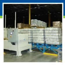
*Load Transfer Stations* An excellent method for transferring loads to captive pallets at the receiving dock.
