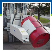
and economical means of handling and dumping drums. Can easily accommodate various drum heights by manually adjusting the top drum stops.
