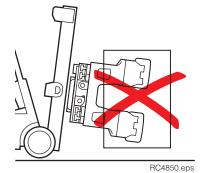
Clamp rolls with pads ahead of roll center and rolls touching the arm kickplate
