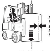
Make sure load is centered and secure prior to lifting and traveling.
