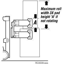
CAUTION: Clamp multiple rolls securely and properly prior to lifting or traveling.
