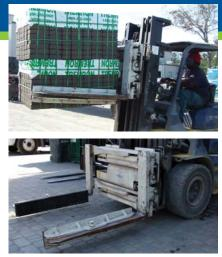
**Brick Block Clamp** Designed to handle concrete building blocks without the use of pallets. Rubber faced articulating arms conform to irregular loads.
