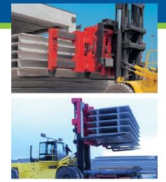
Fork Positioner with horizontal and vertical slewing
