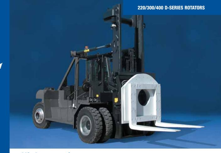
For load inverting and dumping versatility.
