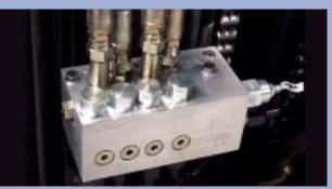
Provides auxiliary pressure relief and flow control to your attachment. Designed for trucks rated 3.5 tons and up. Use in conjunction with the Low Pressure Tank Line Kit.
