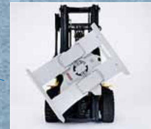
Hydraulically positioned short arm
