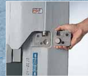
New contact pad mounting with pinless design
