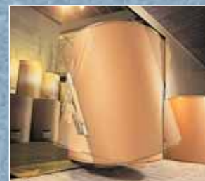
360° rotation allows you to sit roll down in any attitude without concern of truck or damaging roll edge
