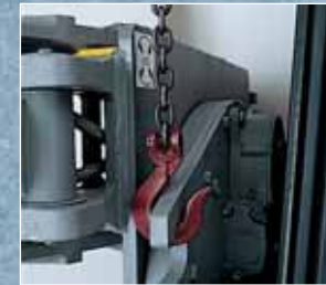
Lifting eyes on baseplate for easy installation
