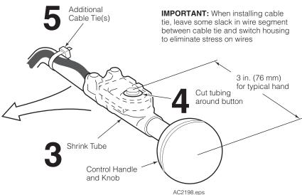
**5** Connect the switch wires to the power supply or truck mounted accessory wires and truck power as marked. Crimp the connectors and cover with the hear shrink tube. Watch for pinch and wear points. Install cable ties as needed.
