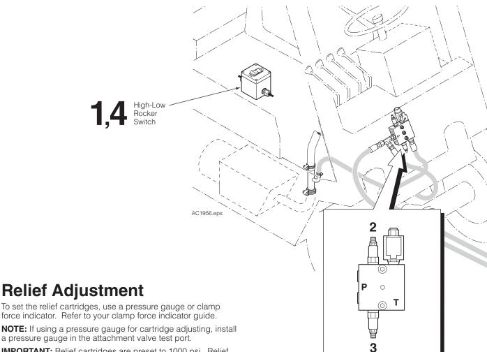
**IMPORTANT:** Relief cartridges are preset to 1000 psi. Relief pressure for each cartridges must be adjusted for your application.
