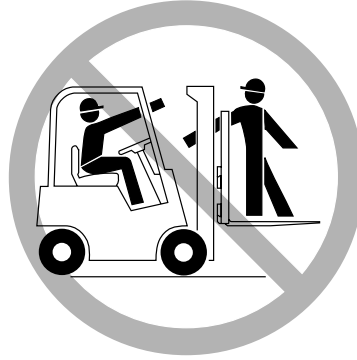
No reach through mast
