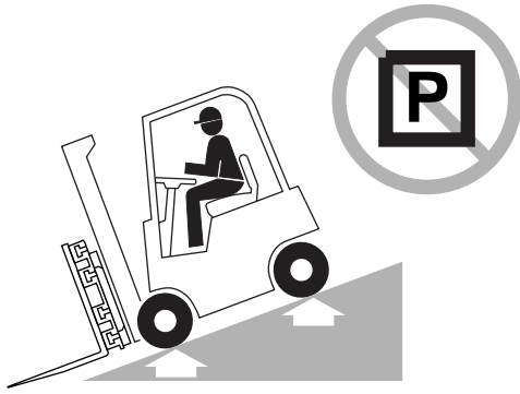
No parking on ramp
