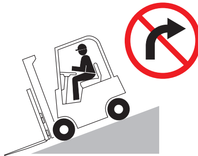
No turning on ramp
