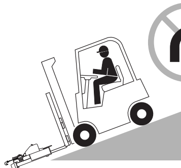
No turning on ramp
