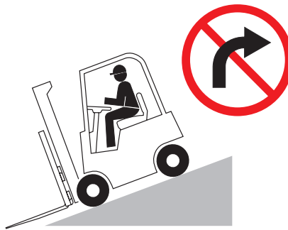
No turning on ramp
