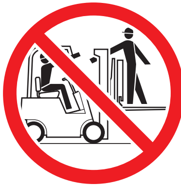
No reach through mast
