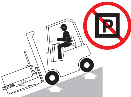
No parking on ramp
