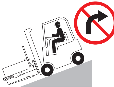
No turning on ramp
