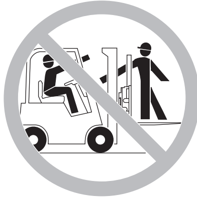
No reach through mast
